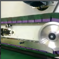
Two abrasive cross belts operating in opposite directions
