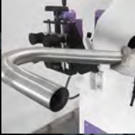
Finishing tight curved tubes with diameters up to Ø76mm
