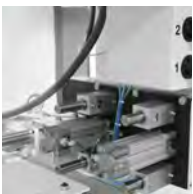
Pneumatic abrasive belt tensioning
