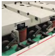
Side grinding stations with vertical oscillation for uniform wear of abrasive belts
