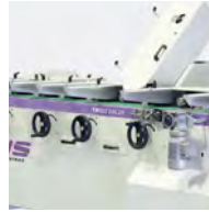
Side grinding stations with vertical oscillation for uniform wear of abrasive belts
