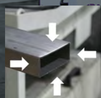
FGW170 8Z: Finishes all four sides simultaneously
