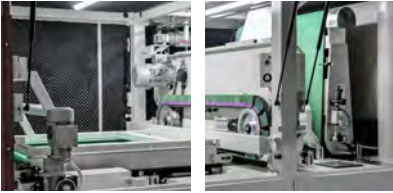
Upper deburring and edge rounding station
