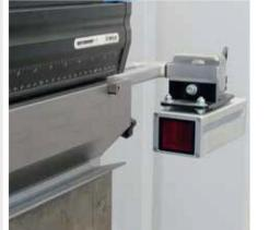
Allows the operator to work safely close to the tools even as the RAM and backgauge moves at high speed.
